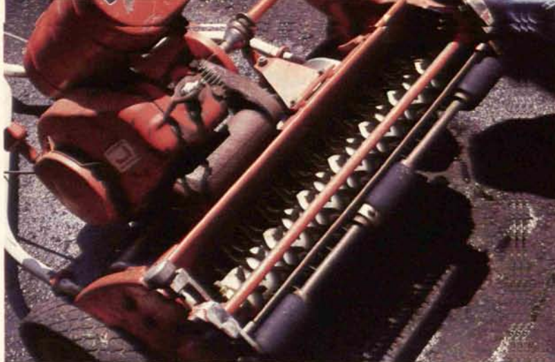
Vertical mowing reels can be used on triplex or single-unit mowers.
