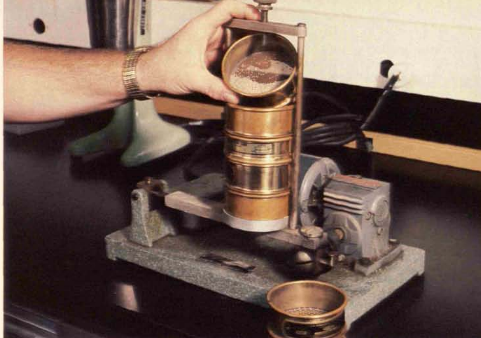
Sieves and shaker used to analyze sand fraction of putting green topmix.
