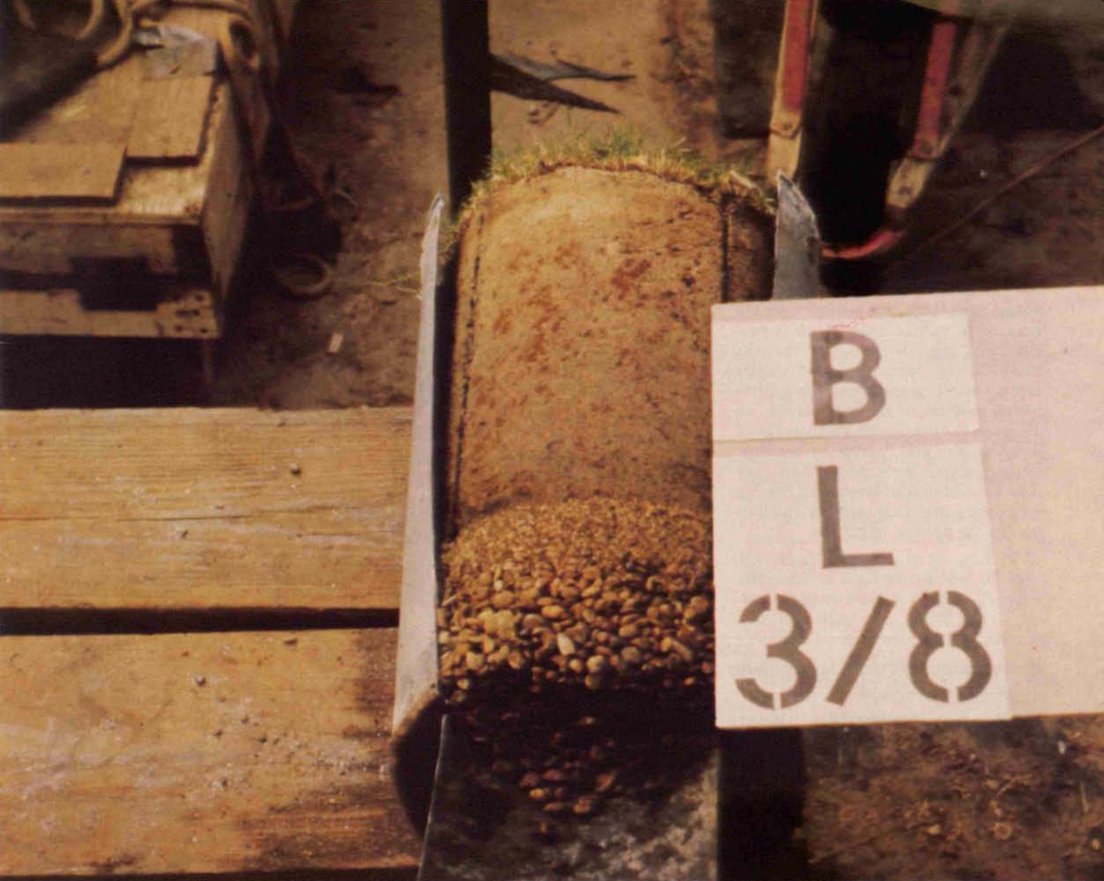
Figure 2. Photograph of the profile of a greenhouse green composed of topmix B overlying a two-inch sand layer over 1 cm gravel.
