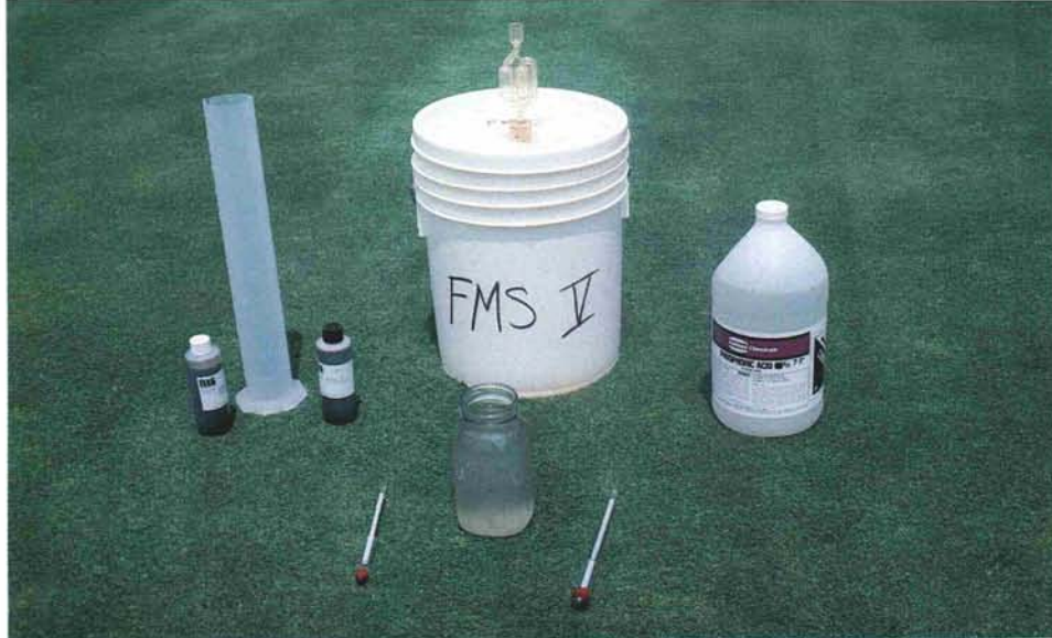
(Left to right, clockwise, starting at top) Enzyme, beaker, yeast, fermentation vessel, acid for pH adjustment, hydrometer, alcohol fuel, and temperature gauge.
