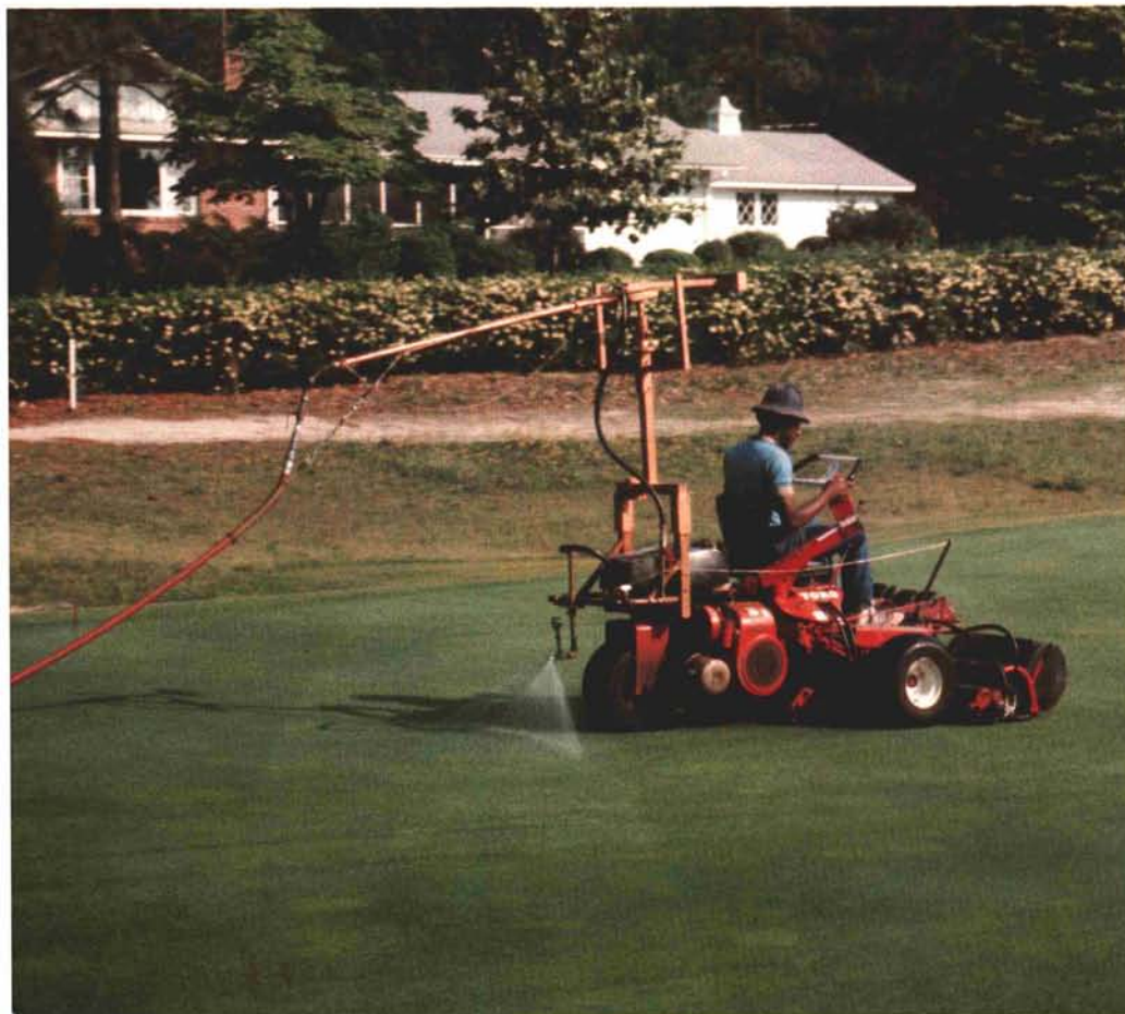
Mowing and spraying greens simultaneously. Regular spray equipment used with extra-long hose. Pine Needles Country Club, North Carolina.
