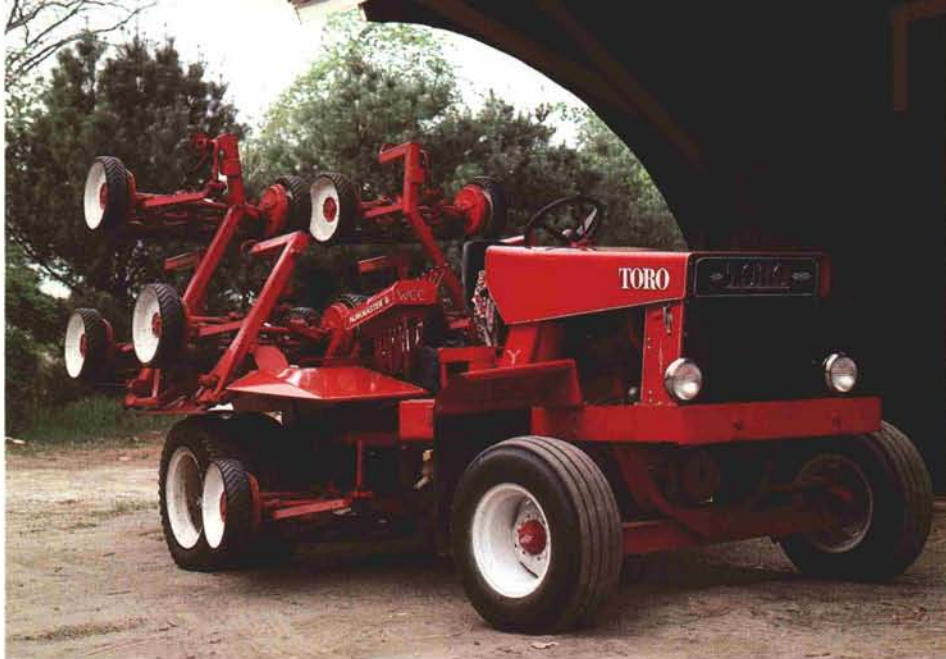
(Right) "Let's cut the rough today!" was the order and, in 1922, this was the easiest way to do it. (Above) In contrast to yesteryear, today's nine-gang unit includes a hydraulic lifting system.
