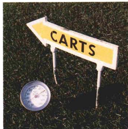
Soil thermometer in position. Golf cart sign protects it from players and equipment.
