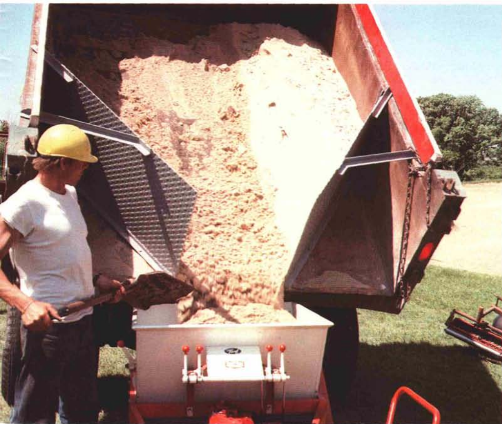
A time and labor saving method of filling the spreader.
