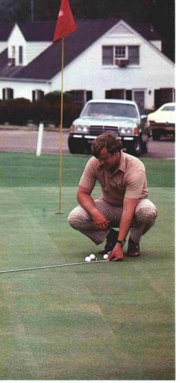
Using the Stimpmeter, three golf balls are rolled in one direction and averaged, then the process is repeated in the opposite direction . . . then the average of the two directions provides the speed of the green.
