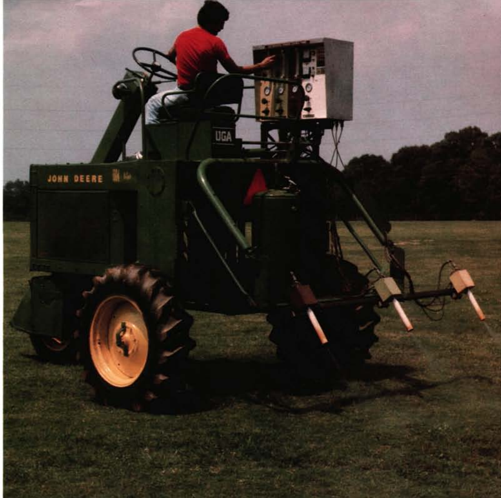
Figure 1. Research prototype machine for evaluating electrostatic pesticide spraying.
