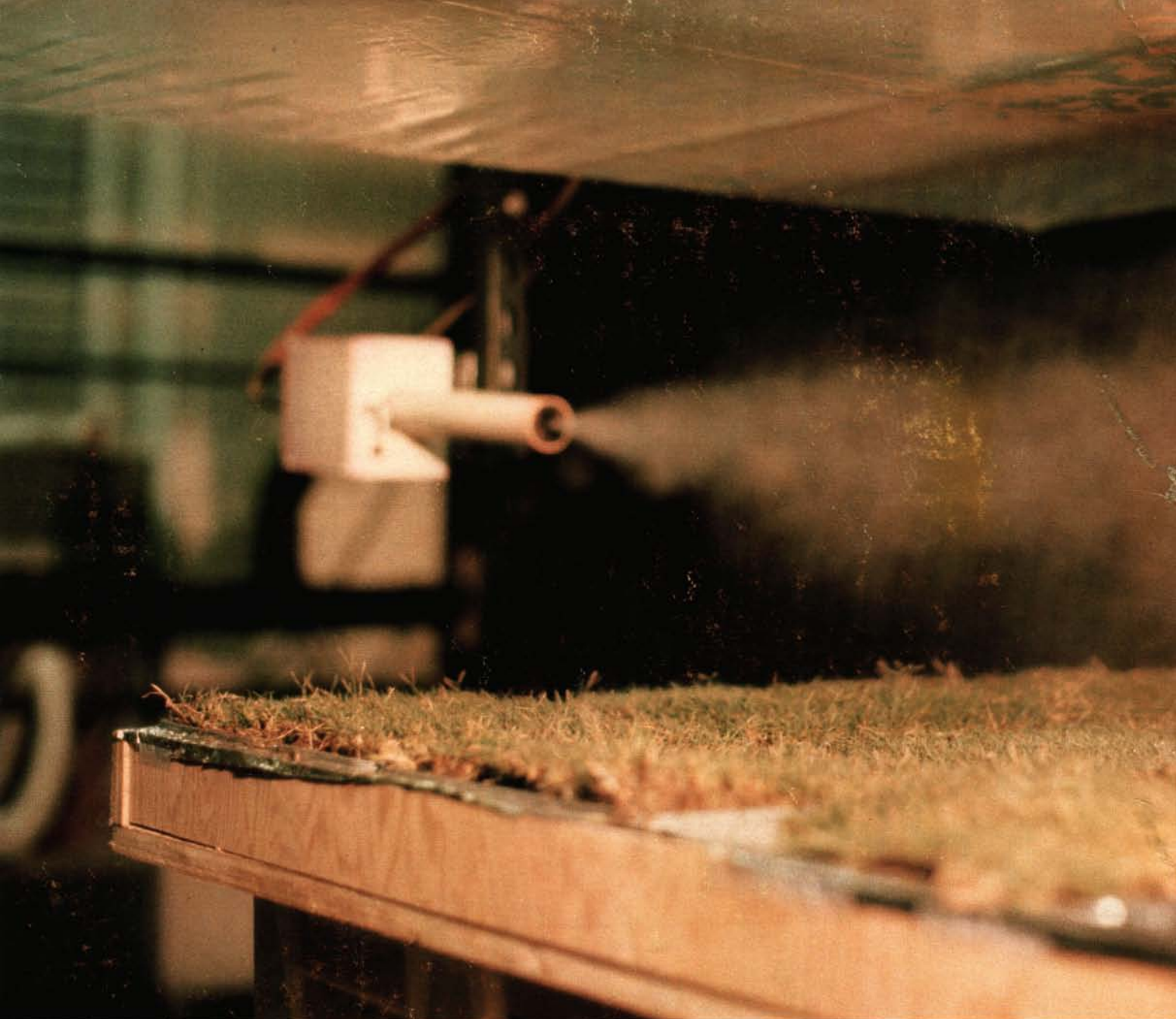
Figure 4. Electrostatic spraying of turfgrass under dielectric-barrier precipitator.
