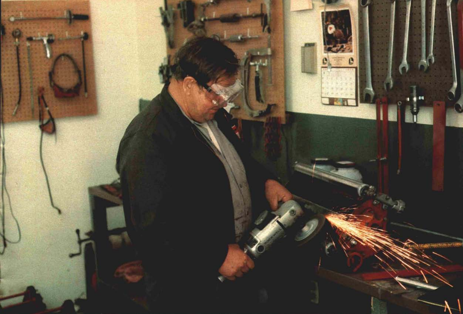
Mechanic James Ames uses a hand grinder to taper front edge of bedknife.
