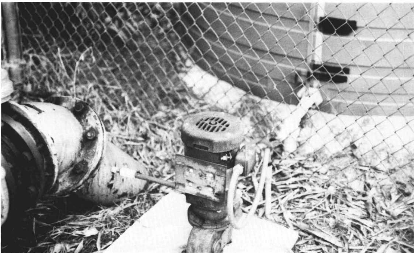
Close-up of the injection pump showing where the liquid fertilizer is injected into the main irrigation line. The black marks on the fertilizer storage tank allow easy determination of how many tons of fertilizer are on hand.
