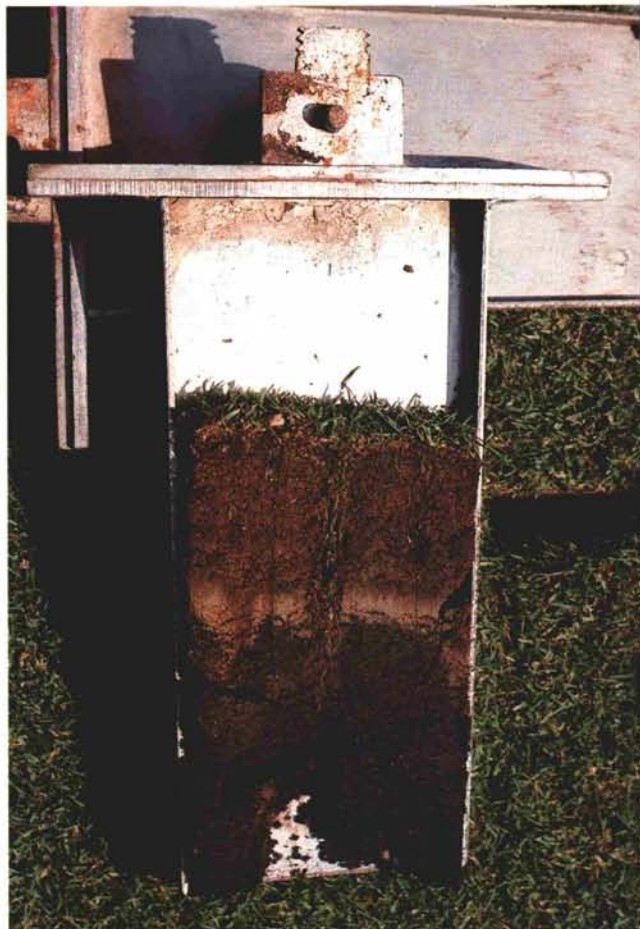
Note clay silt layer through the center of profile, a result of using sod grown on poor soil. The effect is permanent impairment of water movement through the green profile and a soggy, problem green.
