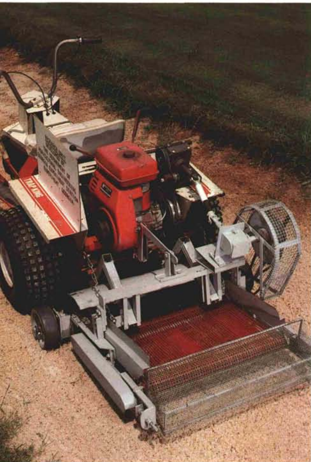
Figure 4. The bunker sand cleaning unit above and the reason why it's needed on the right.
