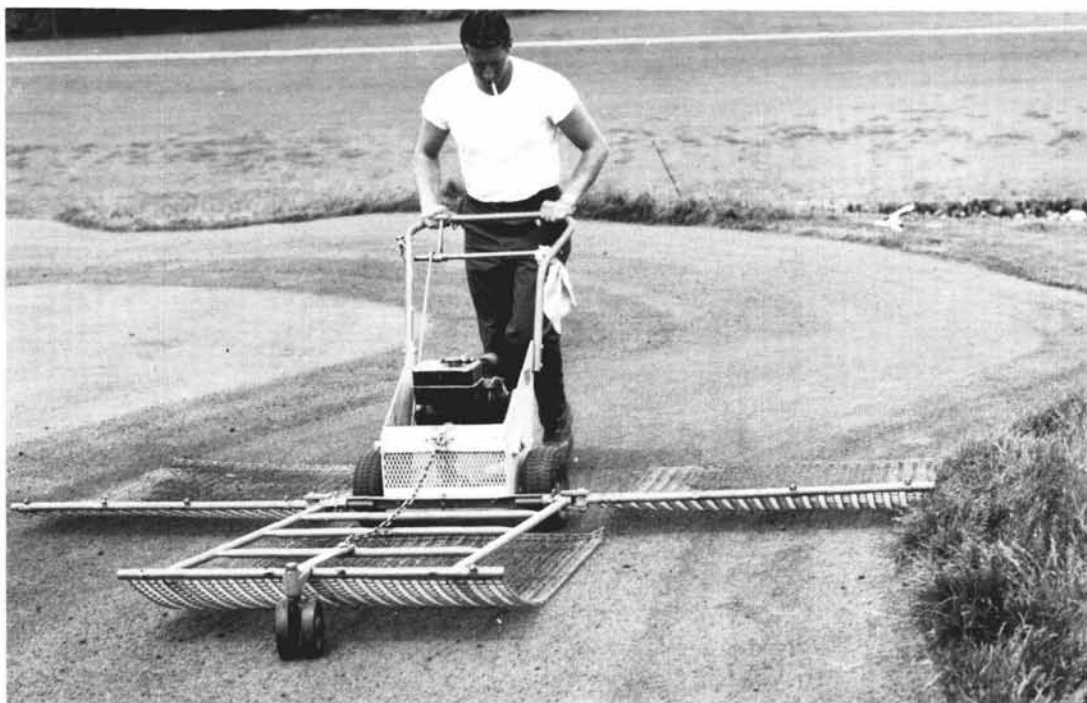
New matting equipment reduces manhour requirements and provides smooth putting surfaces.
