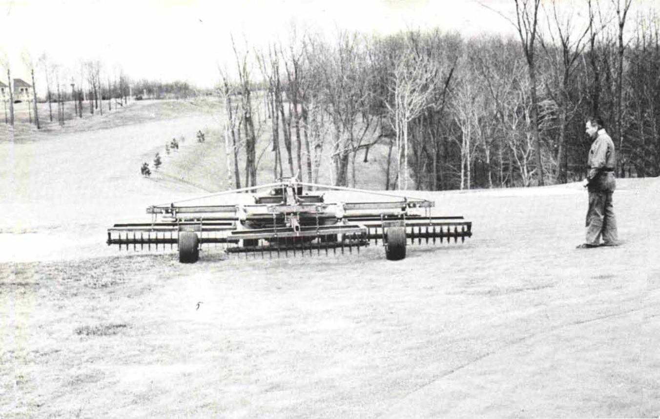
George Ord inspects the spiker he made for fairways, tees and greens.
