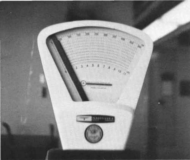
A conversion scale, showing pounds on the bottom and grams on the top. One gram equals the weight of 1 cubic centimeter of pure water at 4° centigrade.
