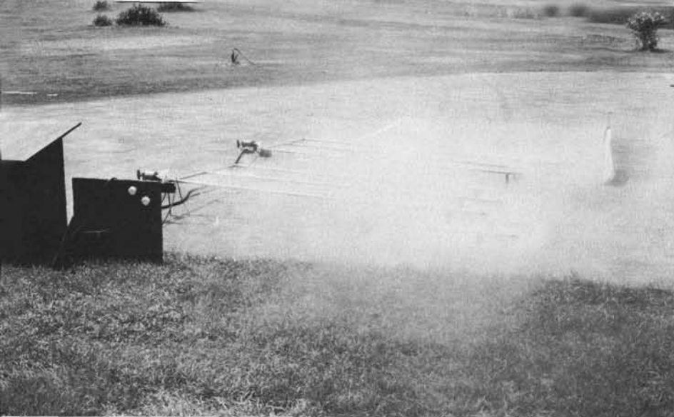
Fig. 2. Light actuated mist equipment with injection of fertilizers and humic acid. Portions of the plastic mist barriers were temporarily removed.
