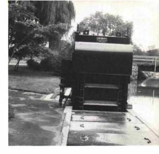
Back view shows continuous rotary elevator and screen which keeps debris out of intake line.
