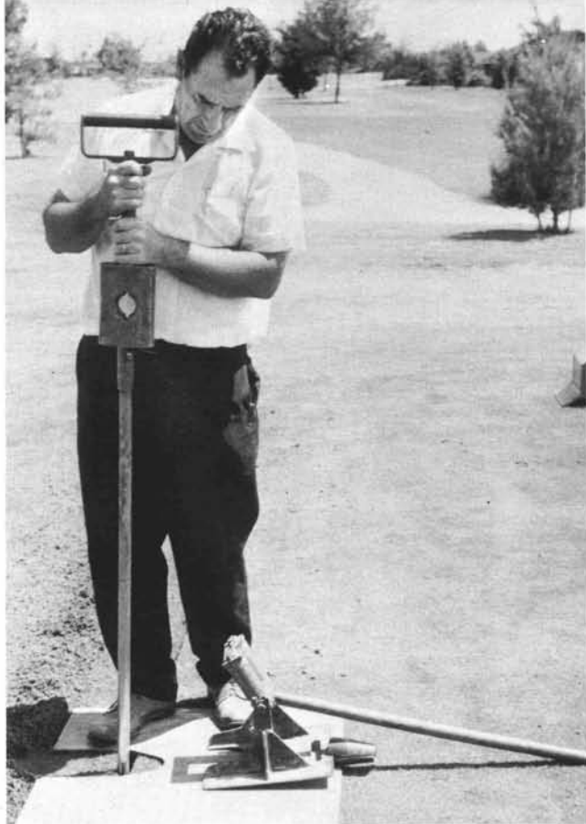
Dr. Henderson at work with a hammer-driven soil sampling tube on No. 2 green.
