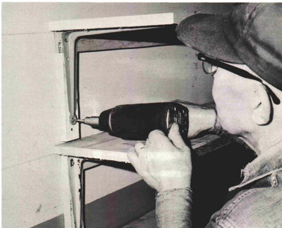
The impact wrench can be used as a screw driver as well as on nuts and bolts.
