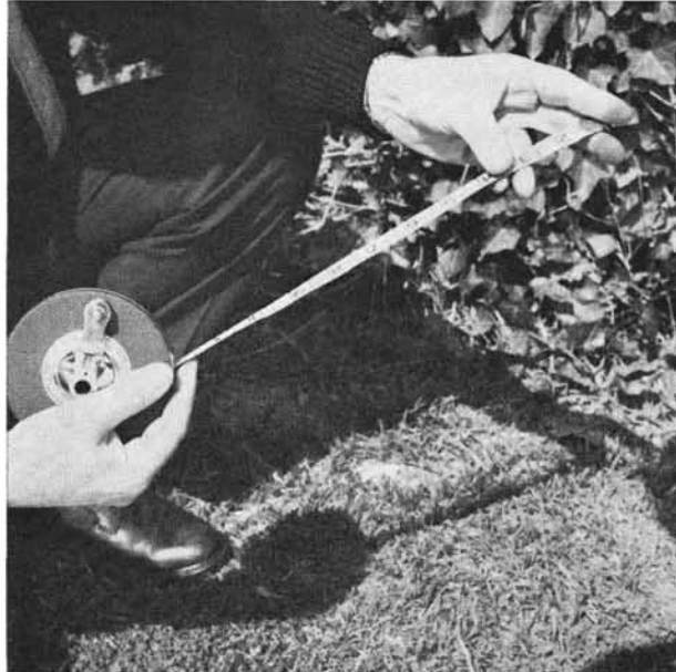
The steel tape, though an arduous task, is still one of the "recommended" methods for accurately measuring the course.
