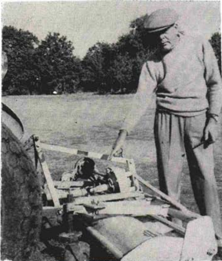
Gen. Winston points to bracket and wheel assembly that he devised to prevent scalping of high spots on fairways.
