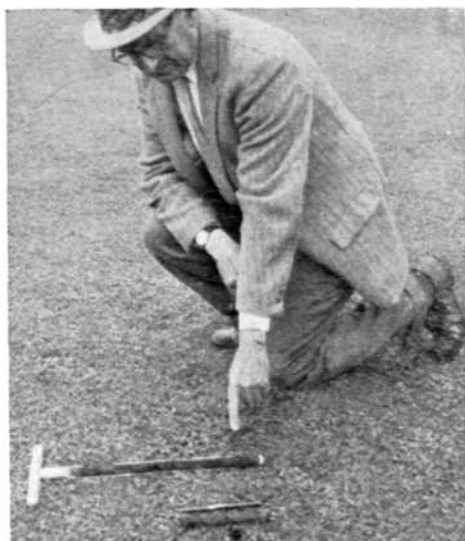
"Molly" Strazza examines soil moisture penetration in a fairway. The soil core removed to a depth of 15 inches indicates moisture present at that depth.
