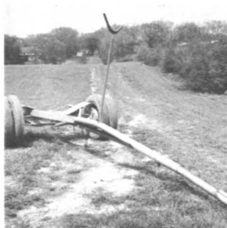
1. A view of the implement which is made of angle iron, pipe, and a dual wheel axle.
