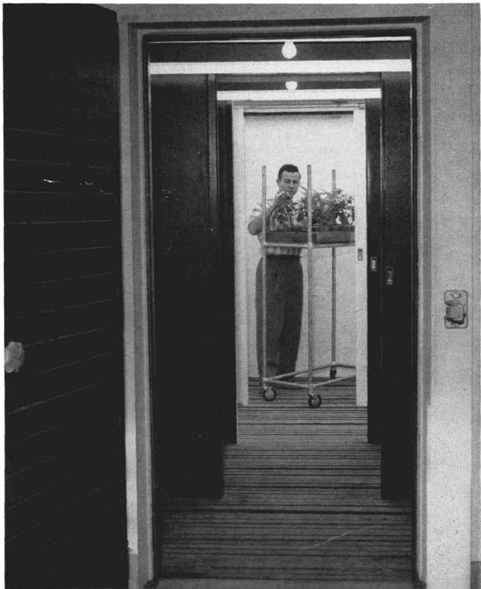
Light tight partitions divide this controlled environment room at U.C.L.A. into four rooms of differing light intensity. Plants are wheeled into the innermost chamber on a specially designed tall cart, made to bring plants near fluorescent lights. In use, outer door and inner partitions are closed.
