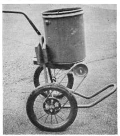
Another pulley wheel was put on the caddie cart inside the right wheel. Both of these pulley wheels are connected by a V belt, so that as the cart is pushed forward the pulleys rotate the horizontal spreader fan, just as the crank did before it was removed.
