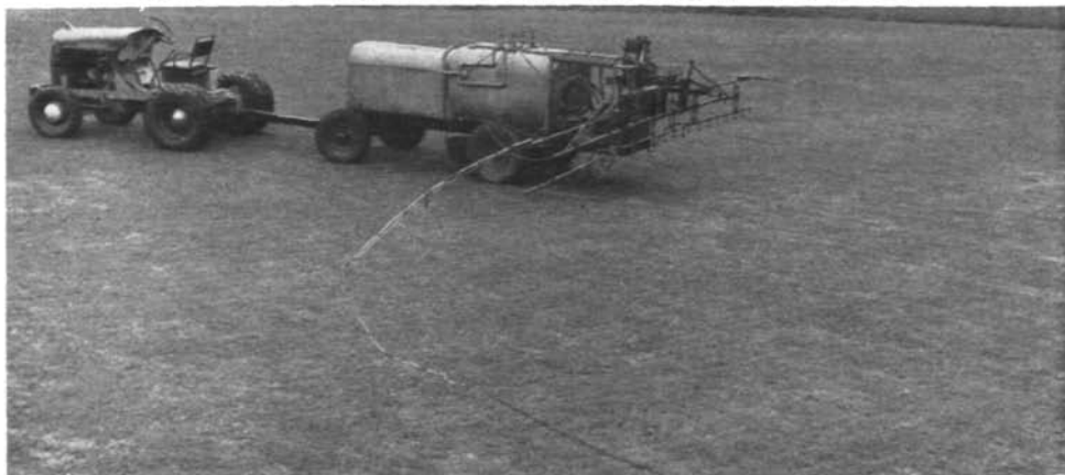
Spray rig at Hercules Country Club, Wilmington, Del., where Superintendent Frank Tull delivers one pound of sodium arsenite to the acre with no skips or overlaps. The trailing marker delivers a slow stream of red dye through tubing from container in center of spray boom.
