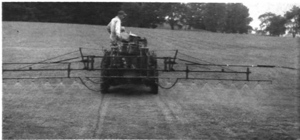
The red dye mark is calibrated so that on the next round the tractor driver puts the left wheels directly on the mark. Weed control with this outfit is done quickly and efficiently.
