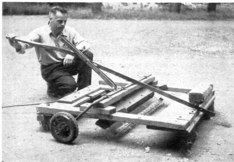
Ellis W. Van Gorder, Superintendent of Stanford University golf facilities, with his home-made device for keeping "grain" and "mat" out of bent putting greens. It has brushes fore and aft with a Del Monte rake section in the center.
