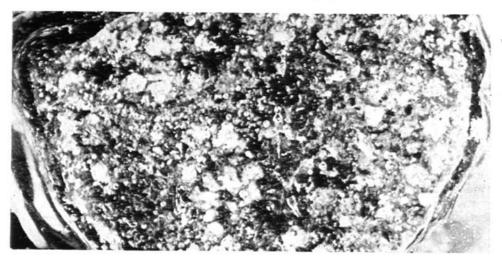
This sample is characterized by a very high proportion of sand which creates a very open pervious structure. There is not enough silt and clay to hold moisture and plant food, necessitating more frequent feeding and watering. A green built on this soil will be firm but will not become compacted.
