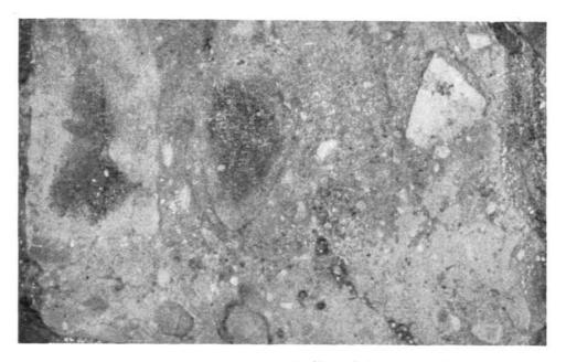
This represents a gravelly clay soil where the films of clay surround the gravel particles, choking off the larger pores and disrupting water and air movement. Less clay and more sand would re-establish drainage and aeration channels.
