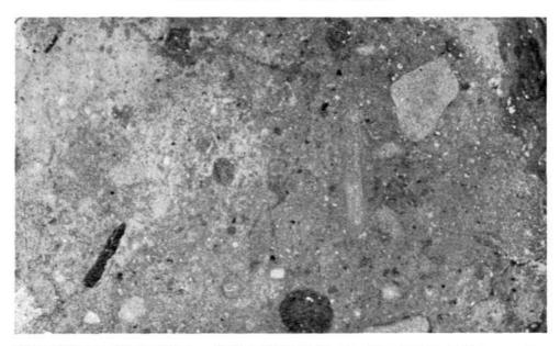
The soil is an extremely dense, light-colored silt loam. The gravel particles are too few in number to provide continuous channels for good drainage and proper aeration. The clay is closely packed around the larger particles. There is not enough sand to create a desirable open porous structure. The dark, irregular-shaped particles are fragments of organic matter.
