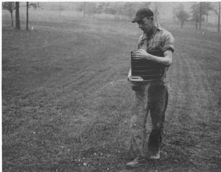
Hand operated cyclone grass seeder which distributes seed by centrifugal action. Such seeders are very useful on small areas such as lawns or roadbanks that are inaccessible to other types of seeders.
