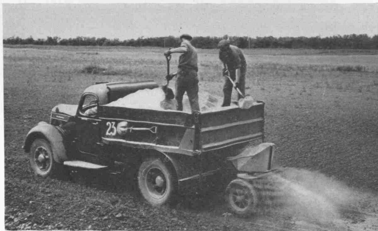
If the addition of lime is necessary before planting, it may be effectively distributed by inexpensive spreaders such as the above which operate behind an ordinary 1 or 1½-ton truck. This machine can be used also for distributing fertilizer and is less expensive than the side-wheel type.
