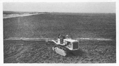
In preparing the seedbed on some soils, harrowing may be necessary in addition to disking. On large areas, this type of spike-tooth harrow may be used to advantage. The comparatively light draft of the spike-tooth harrow makes it possible to pull a large number of units with a relatively small amount of power. The use of such a harrow tends to level as well as to further pulverize the soil.
