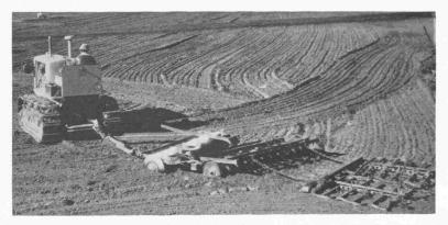
In preparing large areas for turf, a double disk may often be used to advantage. A machine such as this one, having a rear disk which throws the soil in only one direction opposite to the front disk, produces a level seedbed. The spike-tooth harrow dragged behind the disk helps to further pulverize and smooth the soil.
