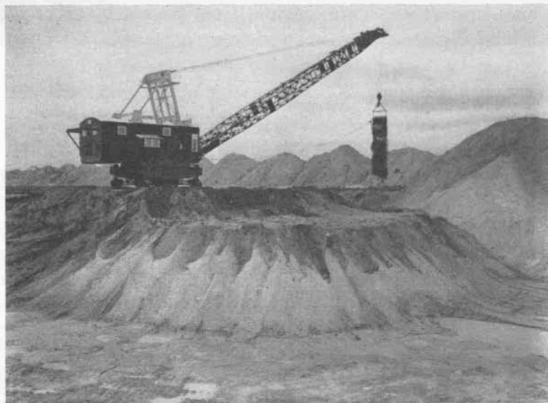
Mining of phosphate rock with dragline in Polk County, Florida.
