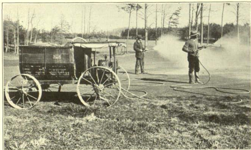
Figure 22.—Fungicides when thoroughly mixed in water can be readily distributed over a putting green in the form of a fine mist by means of a power sprayer and suitable nozzles. Success with this method depends chiefly upon the method of using the equipment.
