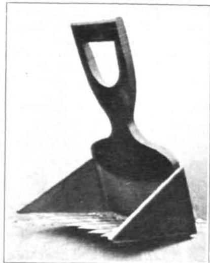
The hand stripper is still used to a slight extent in harvesting Kentucky bluegrass seed
