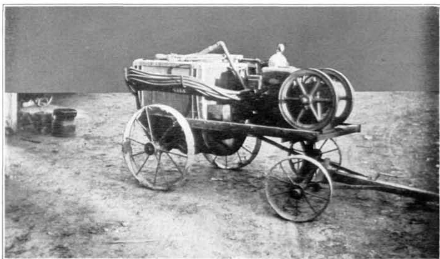
Power sprayer used for the past few years at the Algonquin Golf Club in applying brown-patch fungicides.
