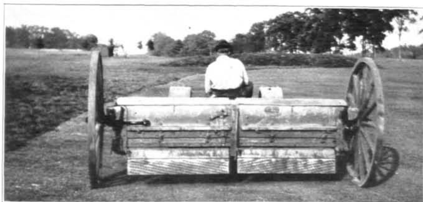
Side and rear views of tractor-drawn fertilizer distributor used at Baltusrol Golf Club for applying a mixture of sulphate of ammonia and cottonseed meal.
