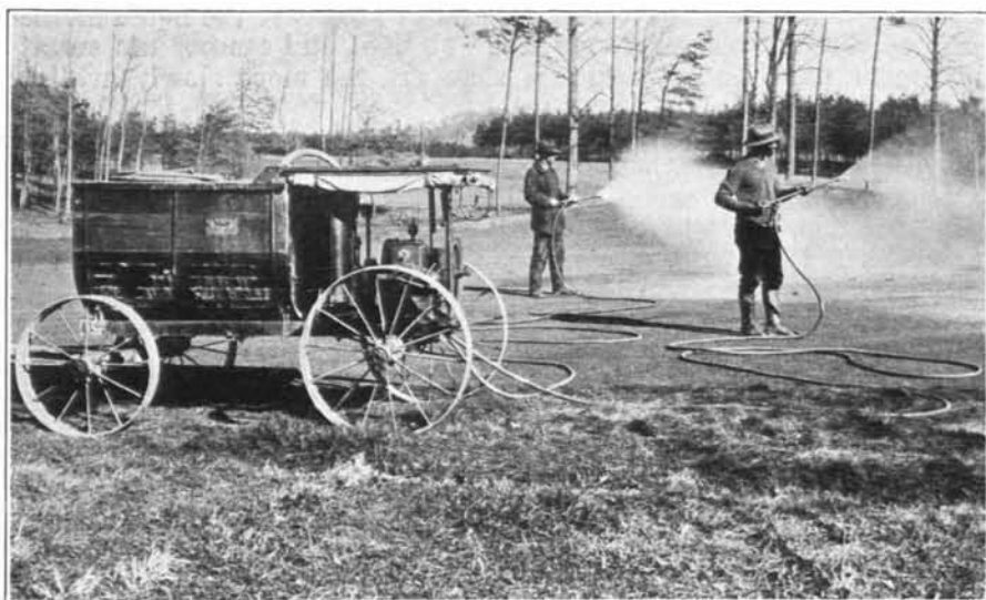
Power sprayer used for applying fungicides and fertilizers at Burning Tree. This machine has given satisfactory results on this course for the past two years.
