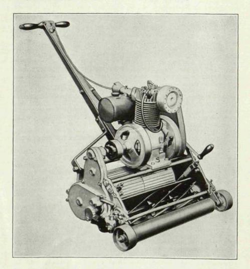
The machine cuts a 19-inch swath. This narrow cut and the compactness of the machine, together with the guard roller in front, enables it to cut undulated greens without scalping the high points. The speed of this machine and the ease with which it is operated enables one man to do approximately the work of two men with hand mowers.
