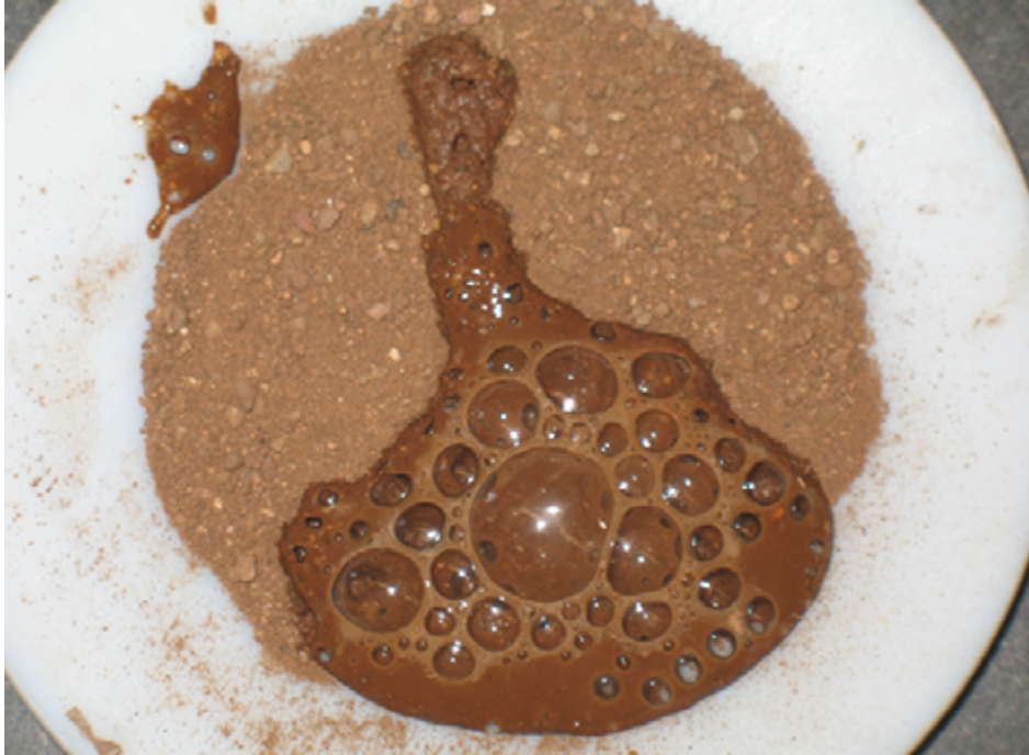
Sulfuric or sulfurous acid applied directly to a calcareous soil creates a reaction whereby lime is dissolved, producing calcium sulfate, carbon dioxide (seen as the fizzing bubbles), and water.
