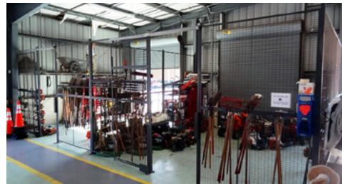
A designated area for hand tools improves worker efficiency as these tools are quickly and easily located each day.
