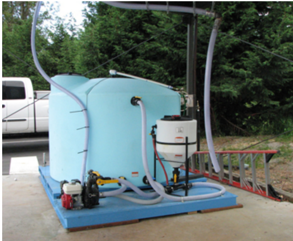
The combination of a large tank (up to 1,600 gallons) and a proportioner allows for rapid spray tank filling and the use of less-expensive macro- and micronutrients.
