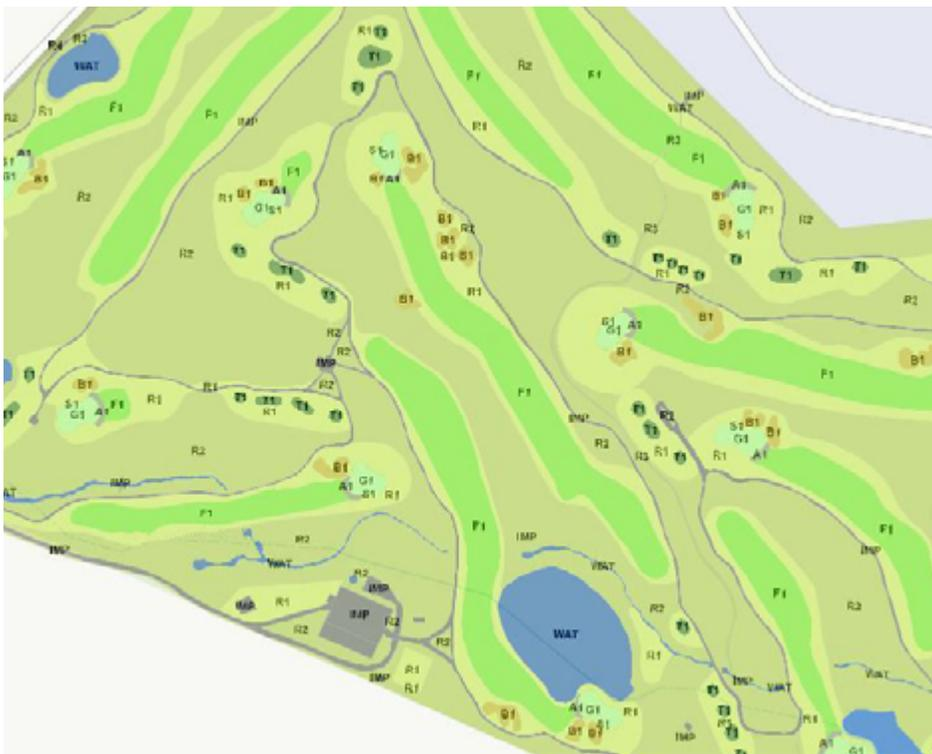
GPS mapping allows turf managers to locate and describe golf course features. Identifiable features can include pest pressure, problematic soil conditions, trees, and underground utilities.
