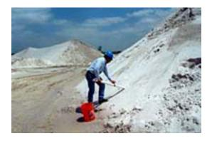
Improper sample collection procedures will result in problems. This sample is being collected incorrectly from the surface of the pile rather than from within the pile. When this sample is tested, the results will not represent the overall make-up of the stockpile. Samples collected in this manner will be highly inconsistent from test to test since the surface of the stockpile changes rapidly.
