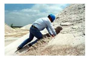
Dig a hole into the face of the pile to prevent collection of any of the sand from the surface of the pile. Expose an undisturbed face of the pile into which the collection tube can be inserted. When you first dig into the pile, material from above will usually flow down the face into the area you are clearing. Keep digging until the hole becomes stable. The shovel also works very well to expose an undisturbed face. Make a vertical cut down into the face just above the sampling point.
