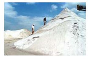
Collect a minimum of 8 samples to ensure an accurate representation of the pile. Take samples at four equidistant points around the pile, at 1⁄3 and 2⁄3 up the face of the pile, for a total of at least eight samples.
