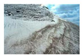
Samples collected from the surface of this pile can vary widely from those collected from within the pile. Notice how the surface of the pile has segregated due to wind and rain. As the finer materials erode, the coarser materials accumulate on the pile surface. Test results of a sample removed from this area would indicate a higher percentage of coarse materials than actually exists in the pile.
