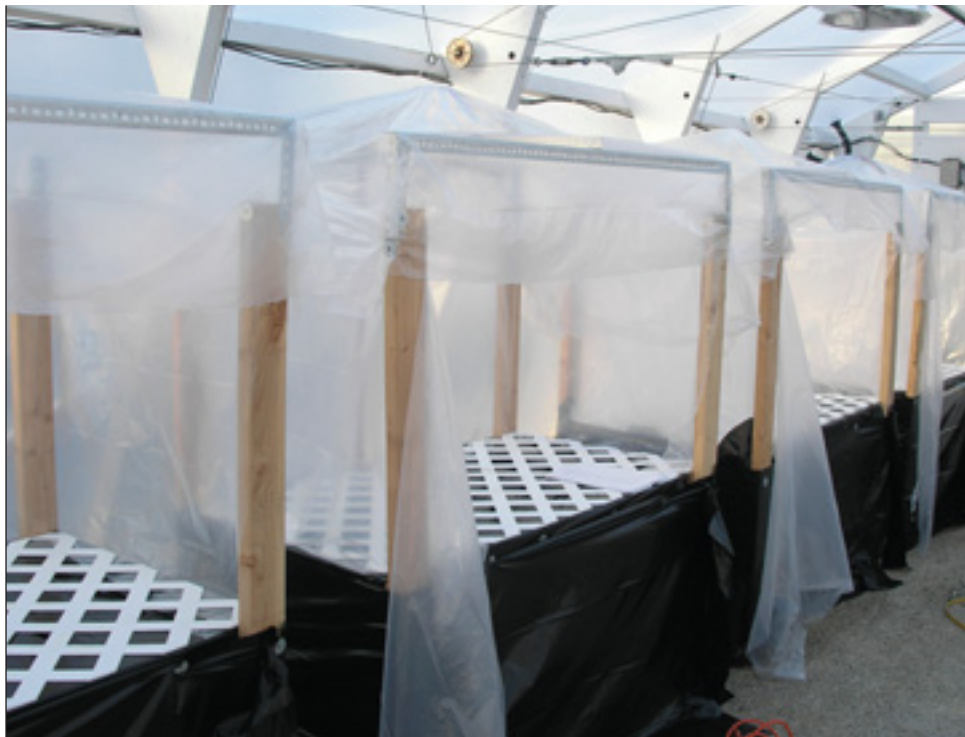
Overhead irrigated salt chambers were built and used to apply salt water to trays containing plants.
