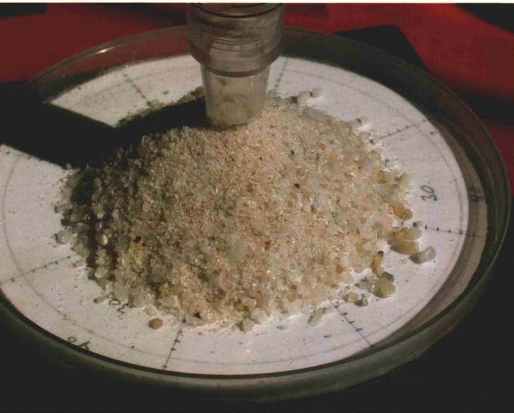
One additional measurement that may help laboratories predict sand firmness is the angle of repose. This measurement is a calculation expressed as degrees, derived from measuring the mean diameter of the base and apex height of a dry sand cone. Coarser textured, more angular sands with wider particle size distribution are more likely to stack higher, resulting in a narrower base and taller cone apex and ultimately a greater angle of repose.
