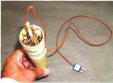
Laboratory-based methods have been developed to measure turfgrass freeze tolerance. Thermocouple temperature sensors are used to measure soil temperatures.
