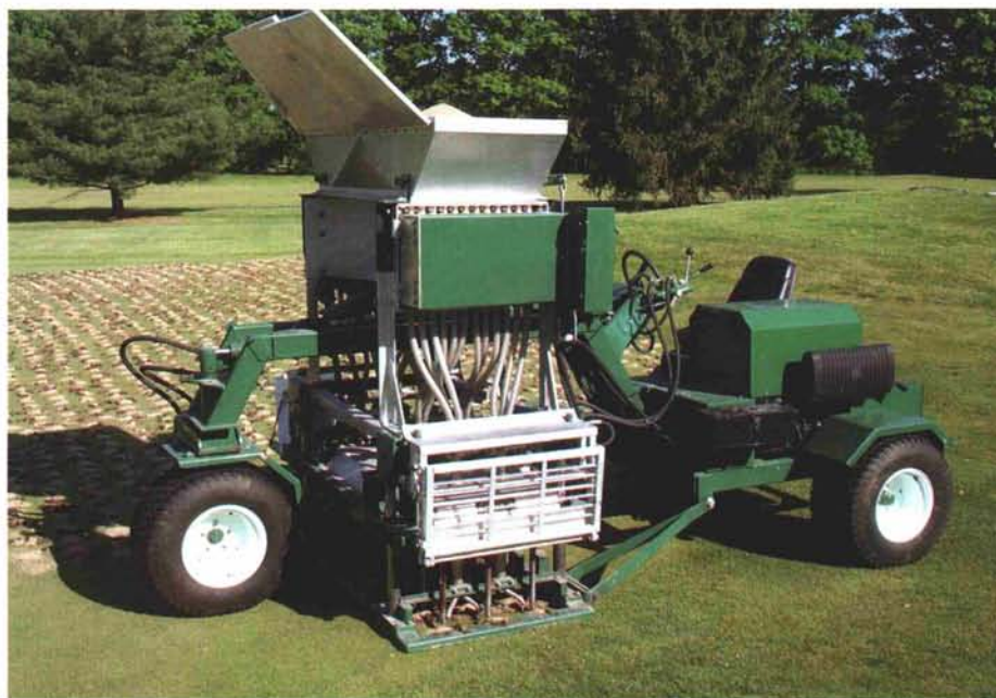
Repeated applications of the deep drill or tine and sand fill procedure usually helps to improve wet greens short of drainage installation or total reconstruction.
