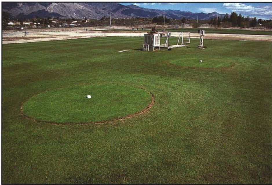
Weighing lysimeters are accurate to within 0.01" per day in measuring actual water use of the turfgrass (ETa) maintained under fairway management conditions.
